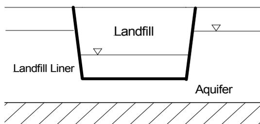
**Scenario 2:** a landfill with a geological barrier and an artificial lining system in a permeable formation.
