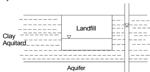
**Scenario 1:** a landfill without an artificial sealing liner in a low permeability formation.
