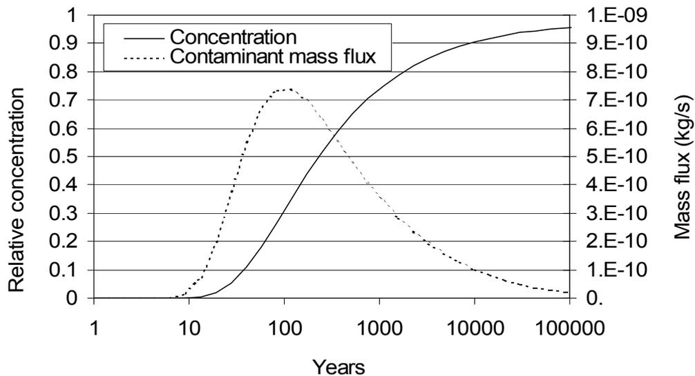
**Figure 13. Breakthrough concentration and contaminant mass flux at the base of a landfill with a compacted clay liner**
