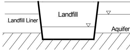
**Scenario 3:** a landfill with a geological barrier and an artificial lining system in a permeable formation but with its base on a very low permeability formation.
