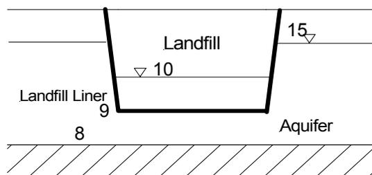
**Scenario 3:** A landfill with a geological barrier and an artificial lining system (including a geomembrane) in a permeable formation but with its base on a very low permeability formation
