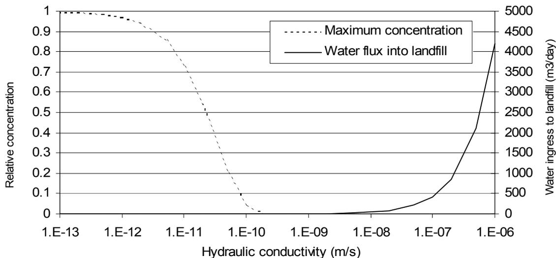
**Figure 12. Trade-off between water influx and contaminant concentration at the liner edge (saturated hydraulic gradient across the liner = 0.2)**
